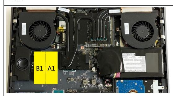
➤ D-side: Channel A DIMM 1, Channel B DIMM 1 For 2x DDR4-2666 sku, A1 and B1 slots on D-side would be empty and reserve for user upgrade.
