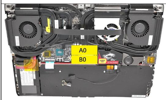
➤ D-side: Channel A DIMM 0, Channel B DIMM 0
