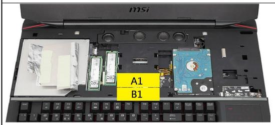
➤ C-side: Channel A DIMM1, Channel B DIMM 1
