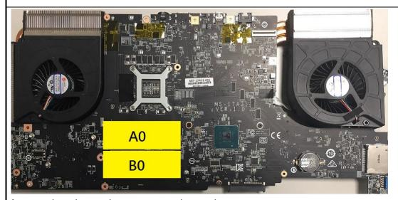
C-side: Channel A DIMMO, Channel B DIMM 0
