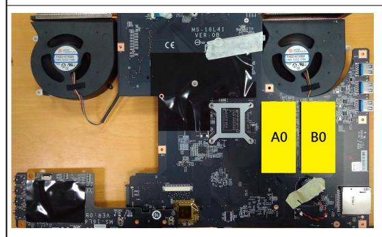
C-side: Channel A DIMMO, Channel B DIMM 0
